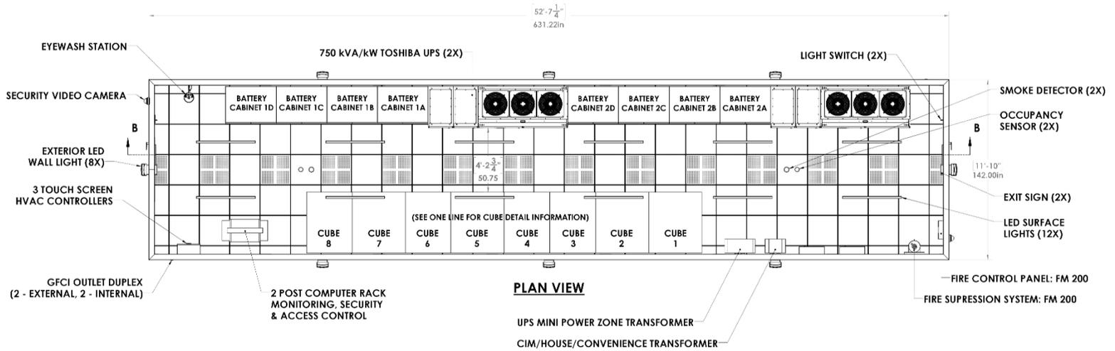
Noted above is a floor plan for a double UPS CIM from a top-down perspective with equipment labeled.
